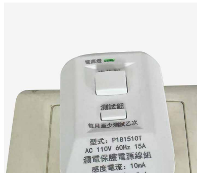
Press the reset button, the green light turns on
