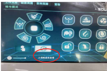
Work head communication abnormality
