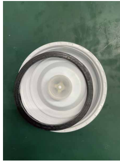
Bucket lid seal is loose
