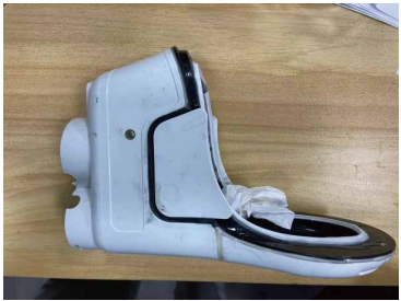
Remove the working head separately for cleaning
