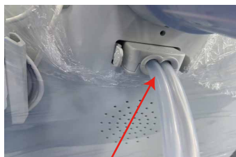
Are the hose joints connected tightly
