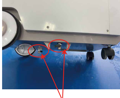
The drain valve is open
