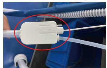
Is the hose signal line inserted in place
